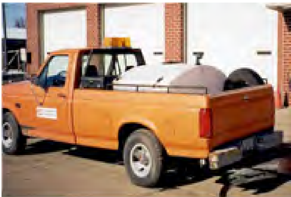
Figure 24: Slip-In Anti-Icing Brine Unit (250 gallon capacity)
