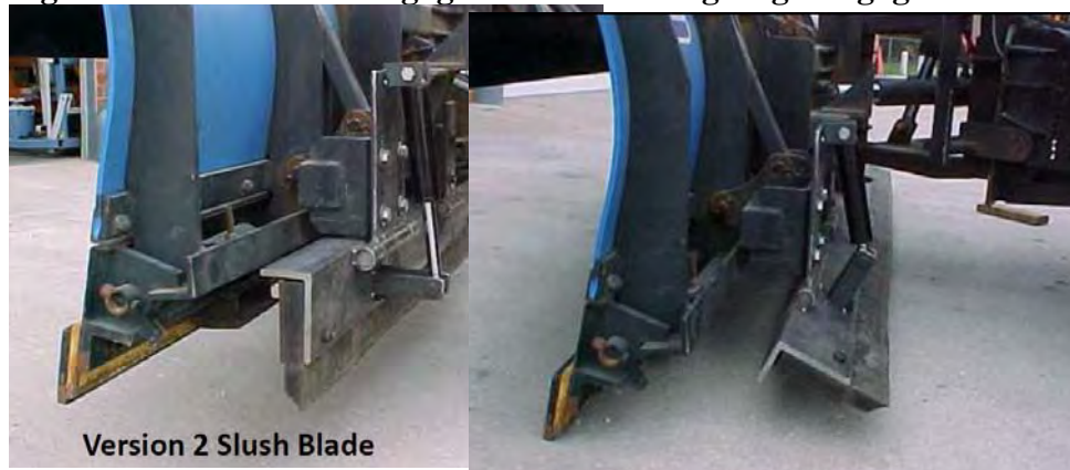
Figure 15. Slush Blade Engaged versus Cutting Edge Engaged
