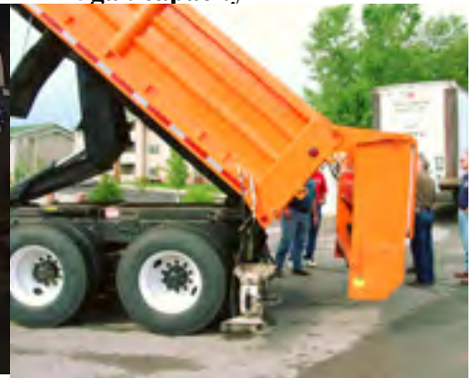
Figure 21. Integrated tailgate 225gal. capacity
