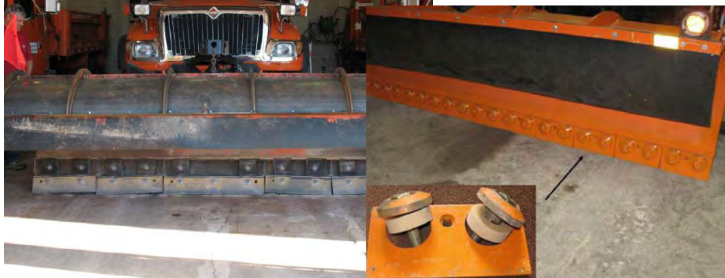
Figure 12. Flexible Edge / Segmented Blade
