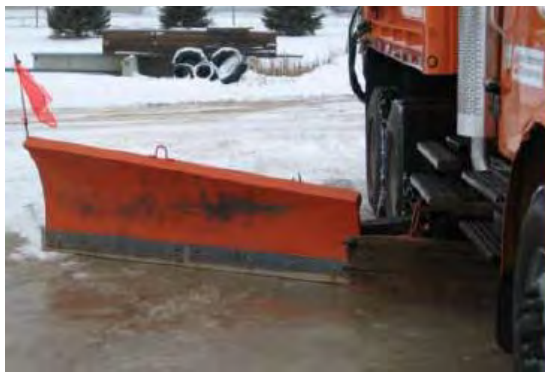
Figure 10. Underbody Plow with Mid Mount Wing Tandem-Axle
