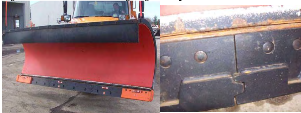
Figure 13. Razor Blade Cutting Edge Set-Up
